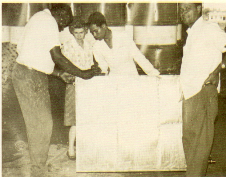
First major trouble came at Paramaribo, Surinam, when this aluminum auxiliary fuel tank ruptured. Repairs took seven days
